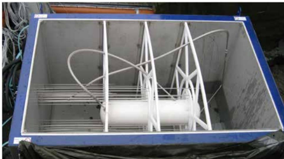
Figure 1: Heat transfer rig with 1 meter long piece of real Snøhvit CO<sub>2</sub> pipeline that can be submerged in variable surrounding medium (photo: Statoil)
