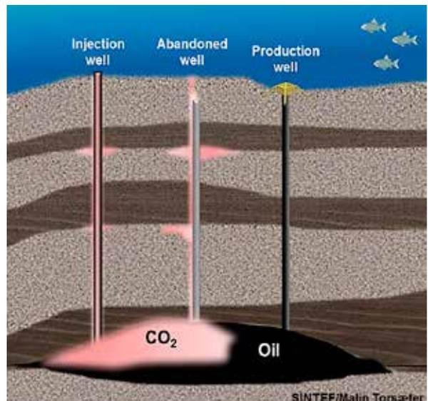
*Well integrity is important for ensuring safe and cost-efficient CO<sub>2</sub> capture and storage, especially if Enhanced Oil Recovery (EOR) is used as an enabler.*
